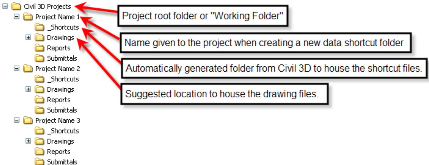
1. Set the Working Folder. This should be the root folder of the project structure. In the example above, it should be the folder called "Civil 3D Projects".
