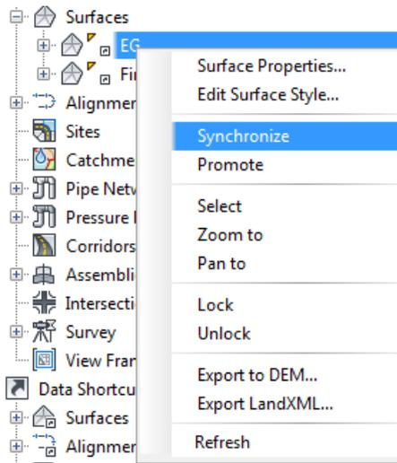
2. Promoting any reference copies the object into the current drawing and removes the link from the source drawing. It can be synonymous with binding an XREF.
