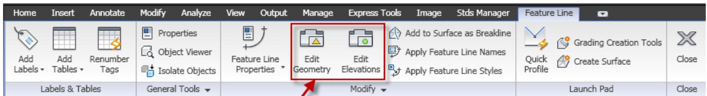
Use these to open the panels in the Feature Line ribbon tab.
