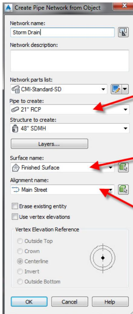
This pipe size is applied to the entire pipe network. You'll have to swap parts manually to individual parts later
